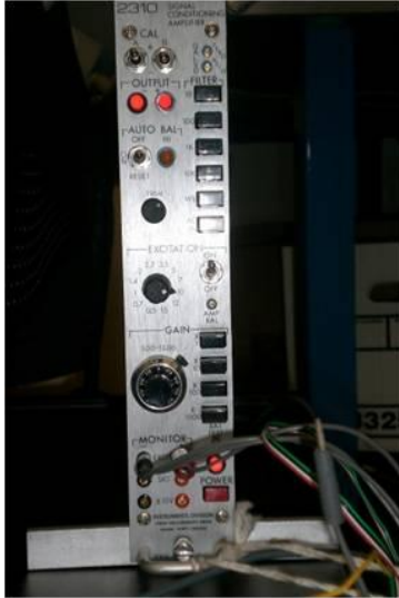
Figure 16 - Load cell power supply
