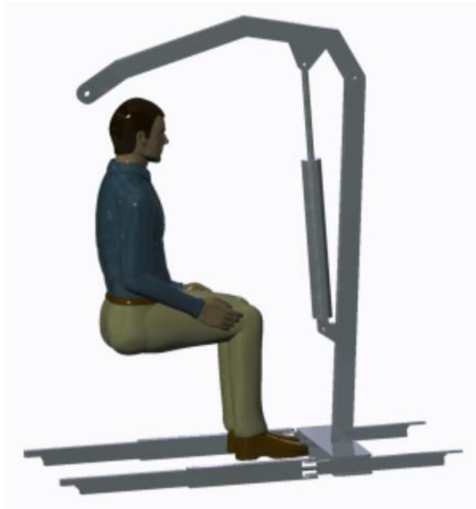
Figure 11: Complete Medical Lifting Design
