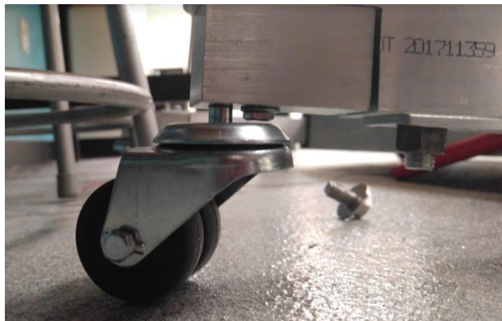
Figure 62: Back Wheel Connected to the Back Wheel Caster
