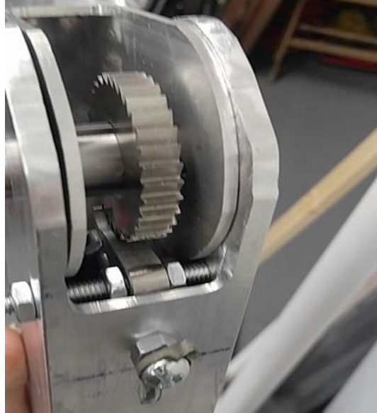
Figure 58: Assembly for the Ratchet Mechanism, Pawl Included
