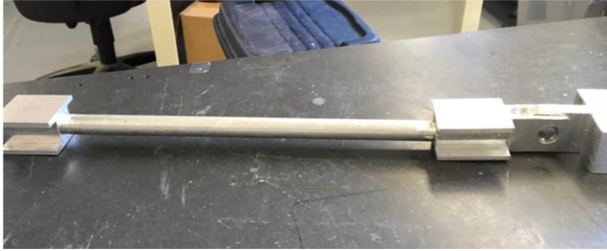
Figure 55: Train Assembly connected to Leg Slider
