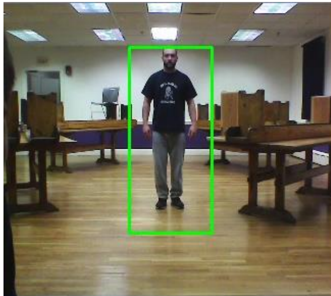
Figure 8: Example of the OpenCV HOG algorithm using the built-in webcam
