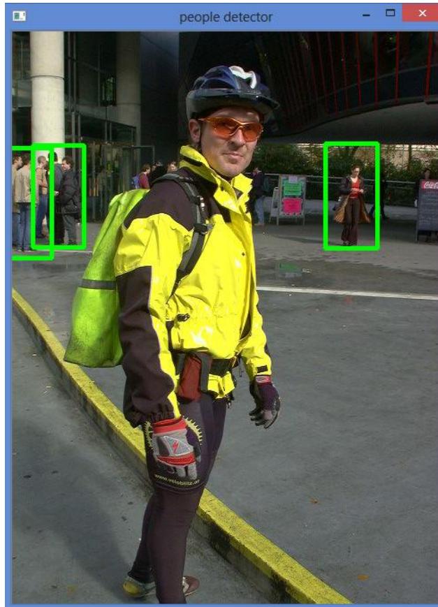
Figure 11: Missed pedestrian in an INRIA image with the OpenCV HOG algorithm
