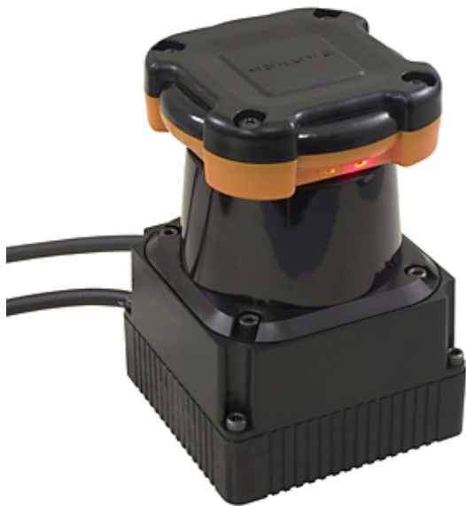
Figure 20 - Hokuyo UTM-30LX LIDAR and specifications
