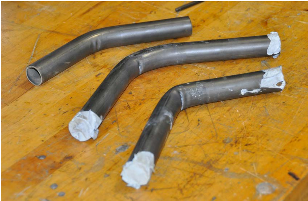
Figure 115 - Example of Kinked tubes
