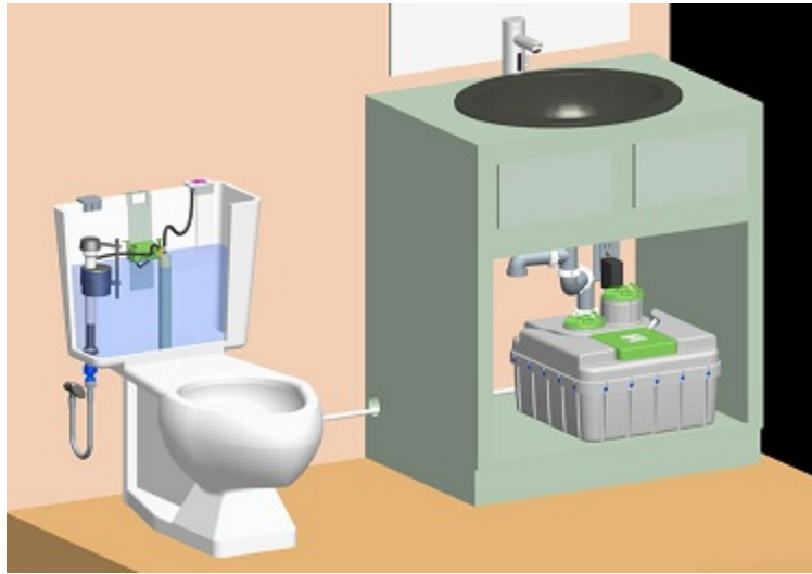
Figure 3: AQUUS greywater system. This figure demonstrates an installed AQUUS greywater system (WaterSaver Technologies, 2009b, para. 2).
