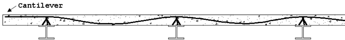
FIGURE 38: WELDED WIRE REINFORCEMENT DRAPING DIAGRAM (CANTILEVER AREAS)
