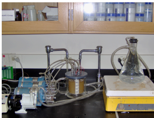
Figure 3.1: The bench-scale bioreactor setup
