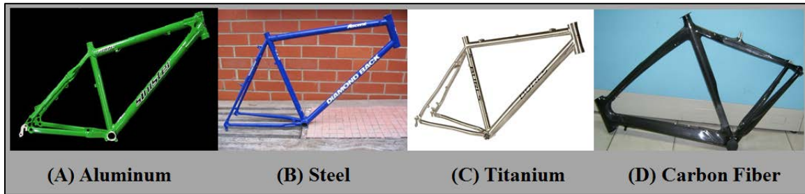
Figure 3: Common bicycle frame materials [20],[37],[21],[43].
