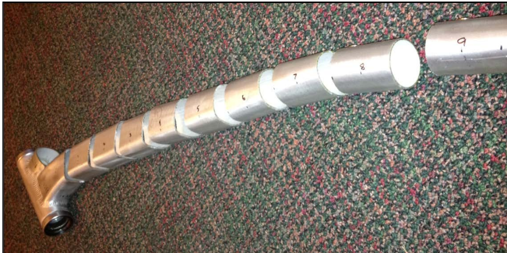
Figure 17: Sectioning of the down tube for cross section measurements.
