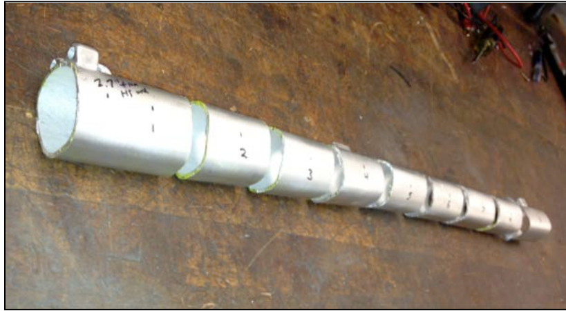
Figure 19: Sectioned top tube for cross section measurements.
