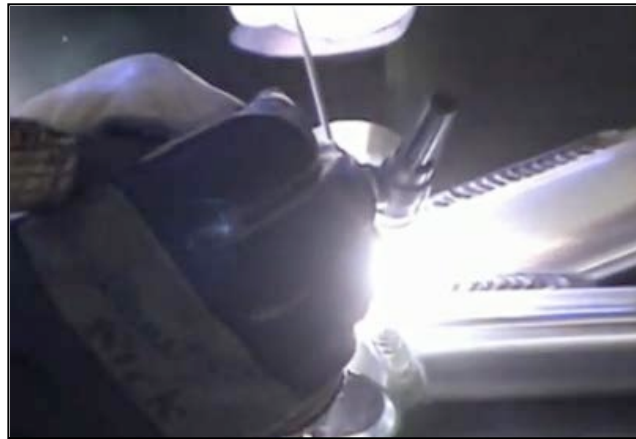
Figure 9: TIG welding the head tube of an aluminum bicycle frame [38].
