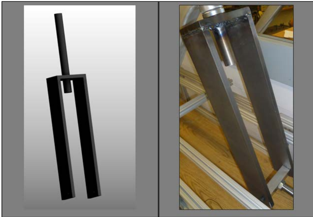
Figure 35: Solid model of test fork and fabricated test fork.
