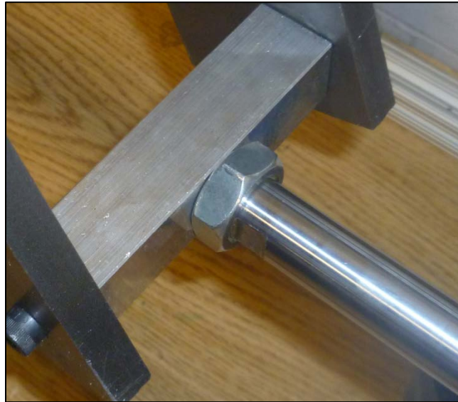
Figure 34: Threaded rod of air cylinder screwed into front dropout.
