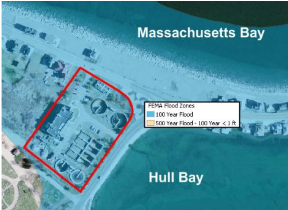
FEMA Flood Zone map for the Hull Wastewater Treatment Plant. The red line indicates the boundary of the facility. (500 year flood – 100 year <1 ft is the combination of the 500 year flood zone and 100 year flood zone under one foot)
