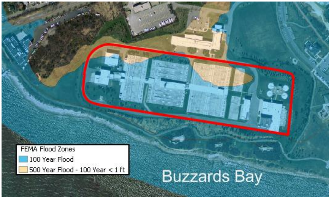
FEMA Flood Zone map for the New Bedford Water Pollution Control Facility. The red line indicates the boundary of the facility. (500 year flood – 100 year <1 ft is the combination of the 500 year flood zone and 100 year flood zone under one foot)
