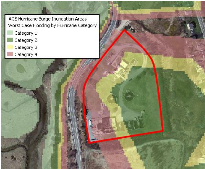
ACE Hurricane Surge Inundation Area map for the Nantucket Wastewater Treatment Facility
