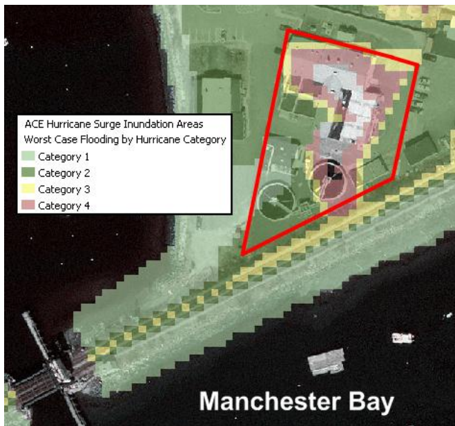
ACE Hurricane Surge Inundation Area map for the Manchester Wastewater Treatment Plant
