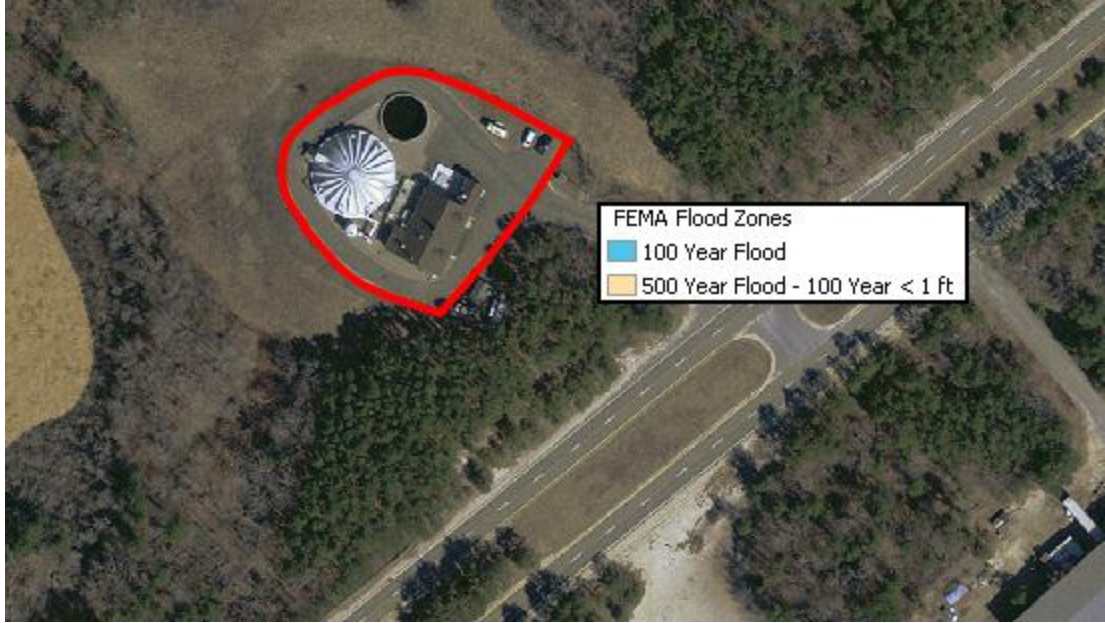
FEMA Flood Zone map for the Provincetown Wastewater Treatment Plant. The red line indicates the boundary of the facility. (500 year flood – 100 year <1 ft is the combination of the 500 year flood zone and 100 year flood zone under one foot)
