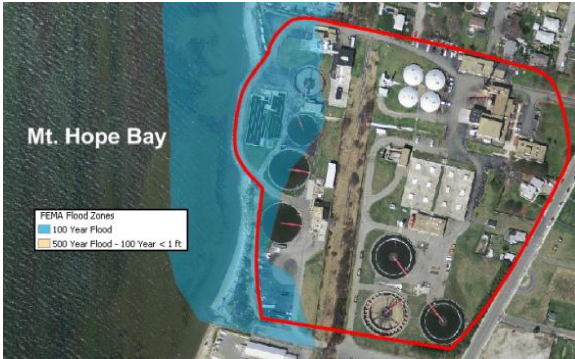
FEMA Flood Zone map for the Fall River Wastewater Treatment Plant. The red line indicates the boundary of the facility. (500 year flood – 100 year <1 ft is the combination of the 500 year flood zone and 100 year flood zone under one foot)
