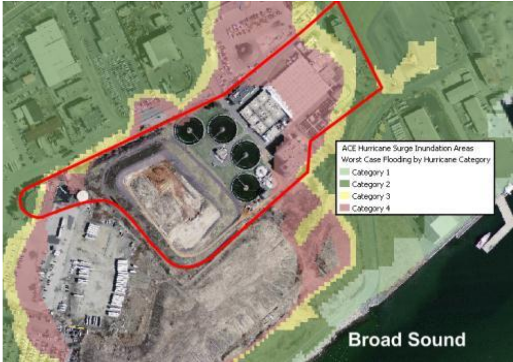
ACE Hurricane Surge Inundation Area map for the Lynn Wastewater Treatment Plant
