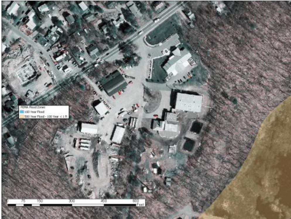
FEMA Flood Zone map for the Rockport Wastewater Treatment Plant. The red line indicates the boundary of the facility. (500 year flood – 100 year <1 ft is the combination of the 500 year flood zone and 100 year flood zone under one foot)
