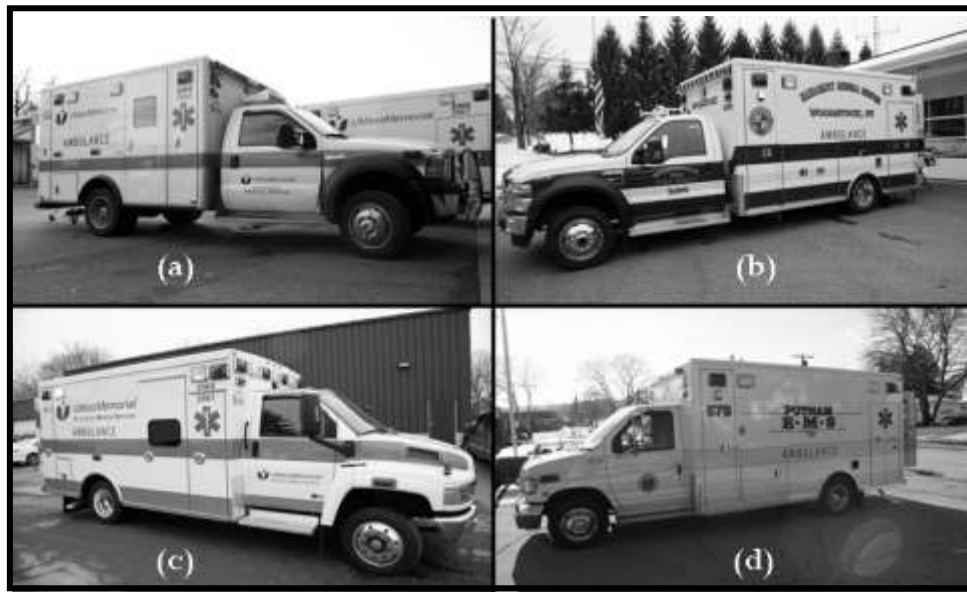
Figure 34 (a-d): Vehicles used in Dr. Cotnoir’s study (a) 2005 F-450 Type I, (b) 2009 F-550 Type III, (c) 2008 Chevrolet C-4400 Type I, and, (d) 2001 Ford E-450 Type III
