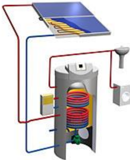
Figure 3-3: SECUSOL Hot water appliance
