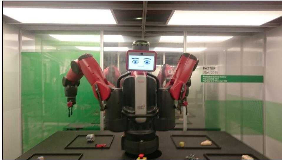
Figure 2.4: Baxter Performing Pick-and-Place Manipulation Tasks (Hull, 2017)
