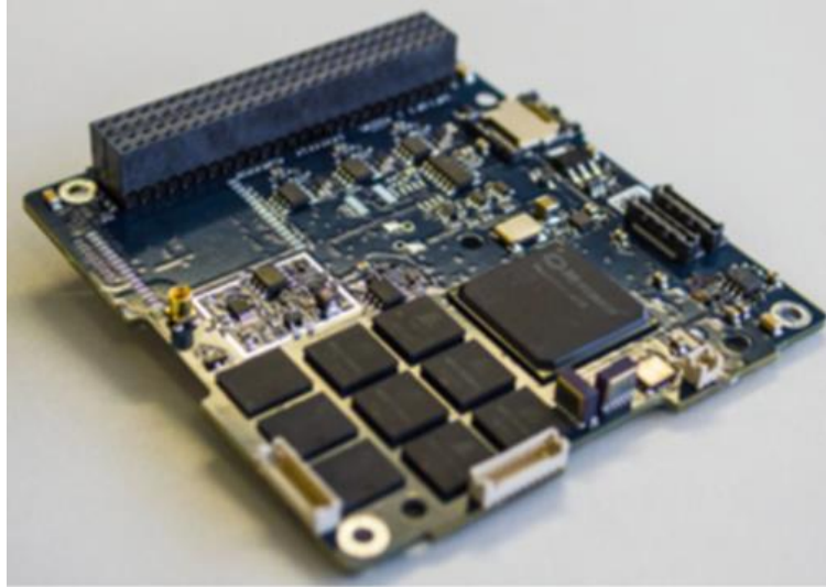
Figure 2: Clyde Space On-Board Computer [14] Copyright 2016 © Clyde Space Ltd.
