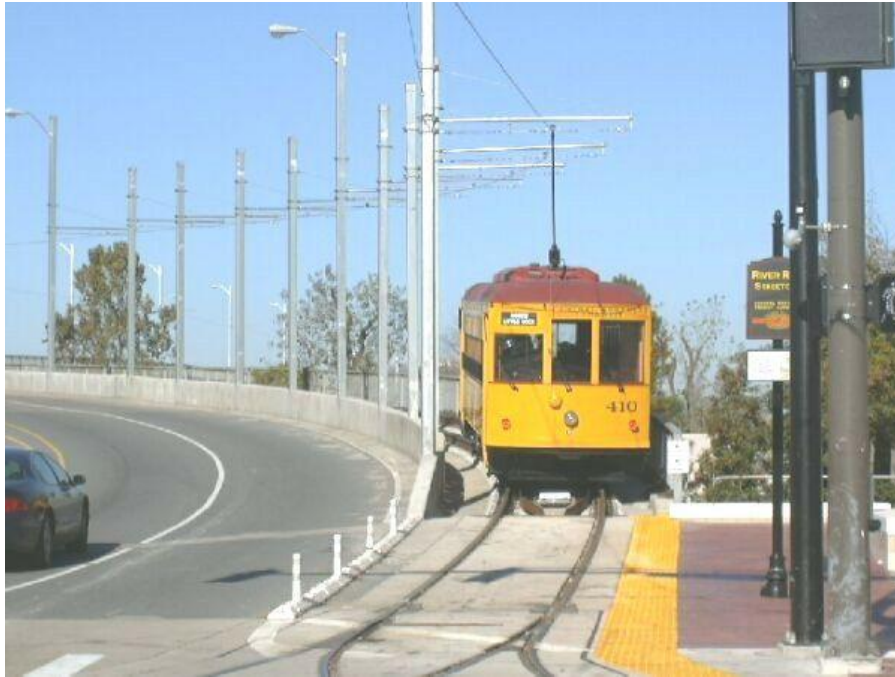
Figure 33 - Light Rail System Appended to Existing Bridge Source: Light Rail Now
