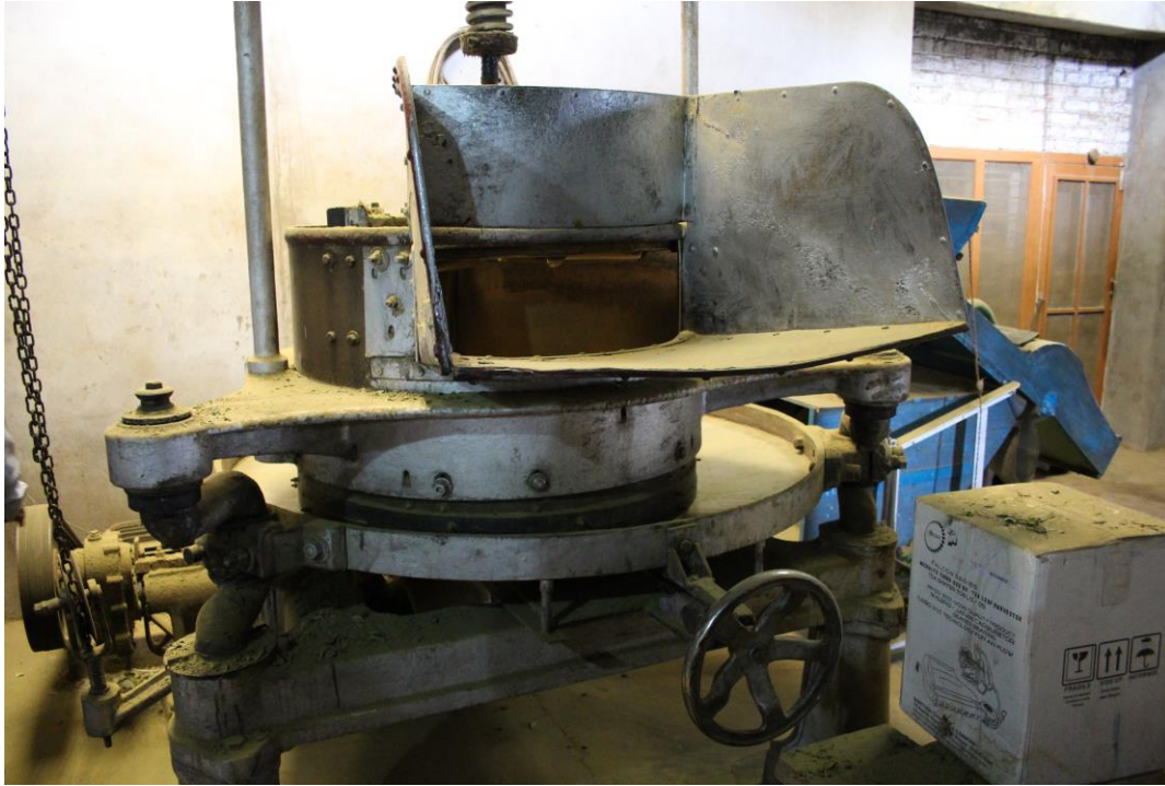
Factories use large rollers to roll several kilograms of tea per batch.
