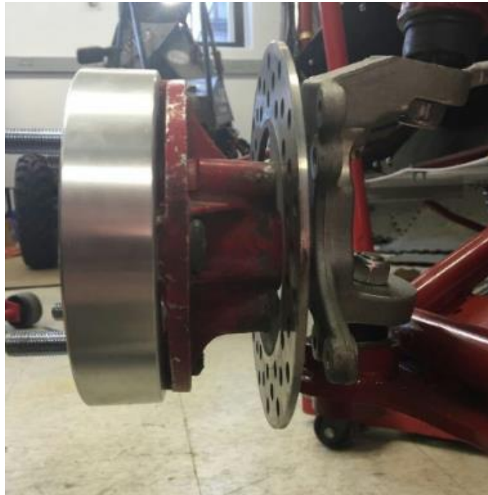
Figure 24: Side View of Wheel Spacer and Hub Assembly
