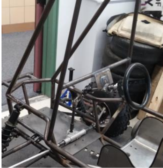
Figure 27: Complete Mounted Steering Column
