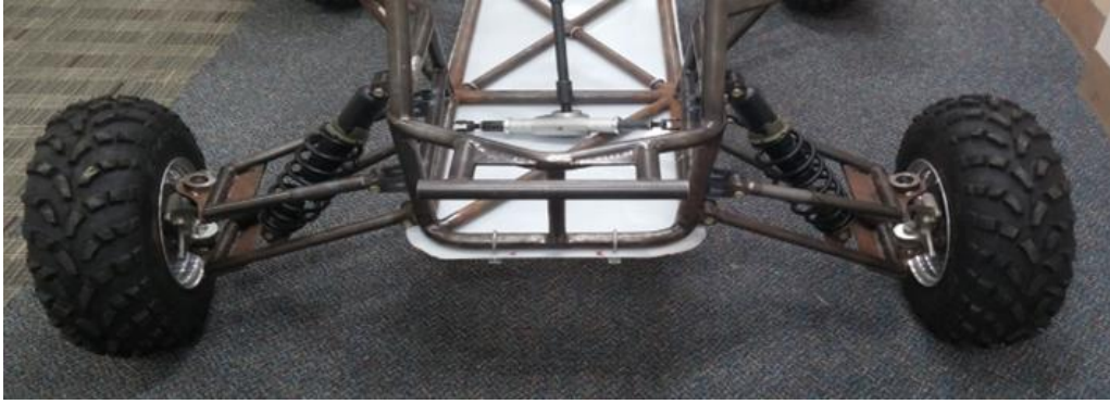
Figure 23: Completed Front Suspension
