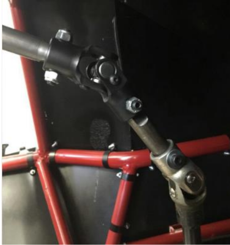
Figure 26: Double U Joint Steering Column Configuration
