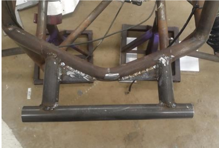
Figure 39: Front Hitch Point Welded by Hubb Equipment
