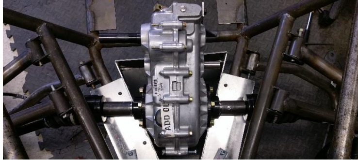
Figure 51: Fitment of Half Shafts with FNR
