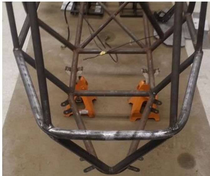
Figure 30: Actual Frame after Hubb Equipment Welding
