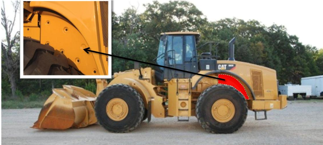
Figure 2: Detailed Location of the Rear Wheel Arch Panel
