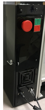
Figure 27: Side of electronics box containing buttons and ports
