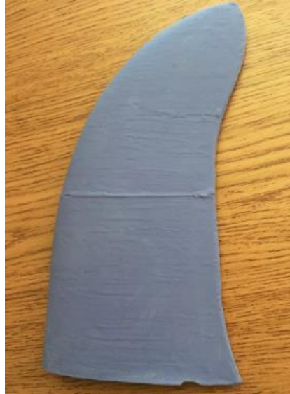
Figure 82: Shore A Harness 45 silicone flexible flipper
