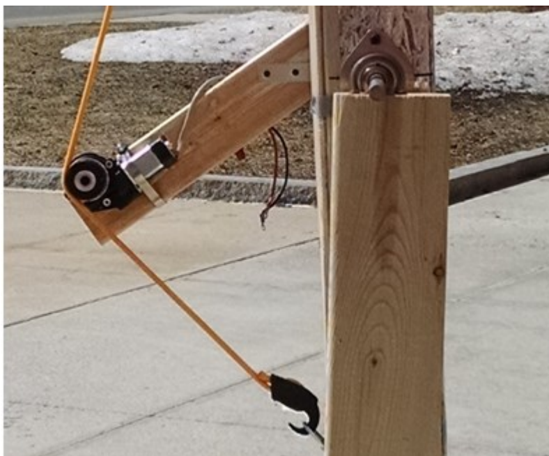
Figure 68 Mounted Electric Motor
