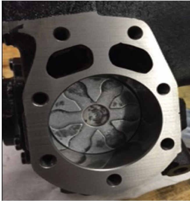
Figure 51 Ground down engine-to-head surface
