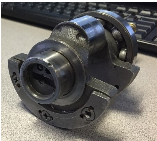
Figure 11 Crankshaft prior to being ground down
