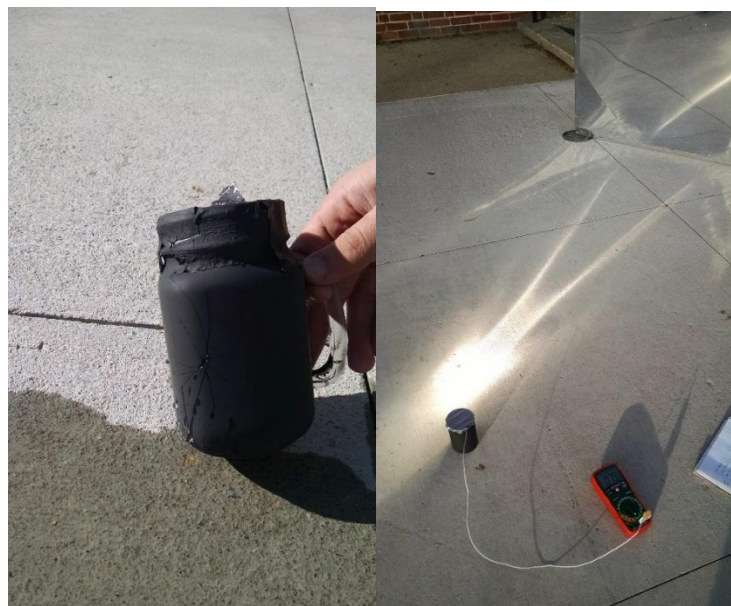
Figure 44 Setup for Black painted glass jar testing
