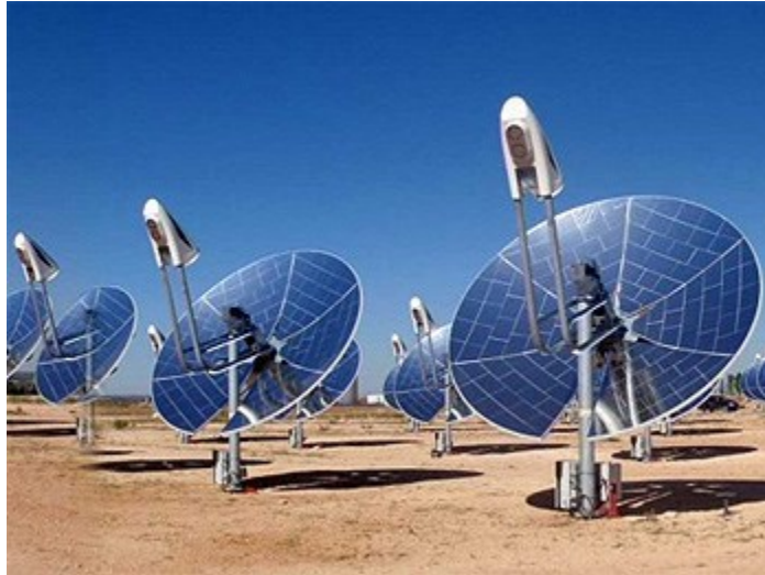
Figure 8 Infinia Stirling Engine Solar Array ("30kW Maintenance Free Stirling Engine for High Performance Dish Concentrating Solar Power, 2010)
