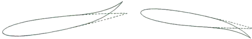
Figure 31: Extended span of flexible foils (solid) compared to rigid foils (dotted), adapted from [45] 15
