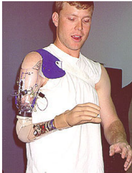
Figure 13 - Example of a Myoelectric Upper Limb Prostheses
