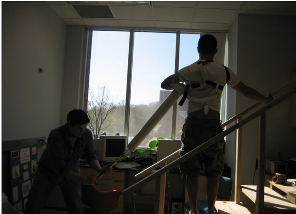
Figure 106 - Axial Load Test at -45°
