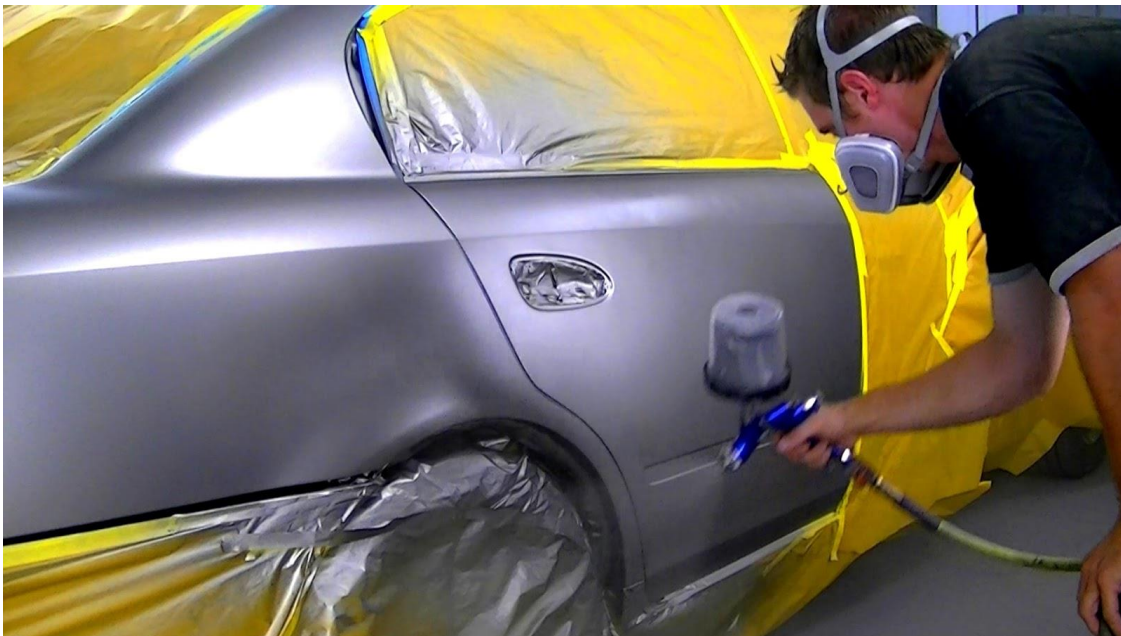
Figure 1: Photo of the automotive painting style/technique called "blending" [1]
