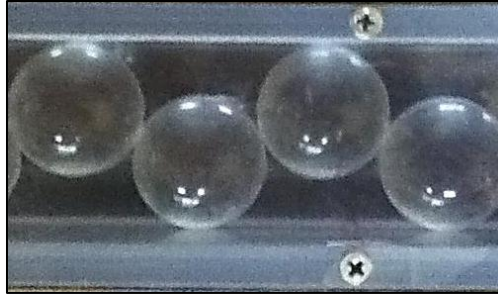
Figure 5: Bottom-Packed Channel Physical Packing. Above: Side View. Below: Top View
