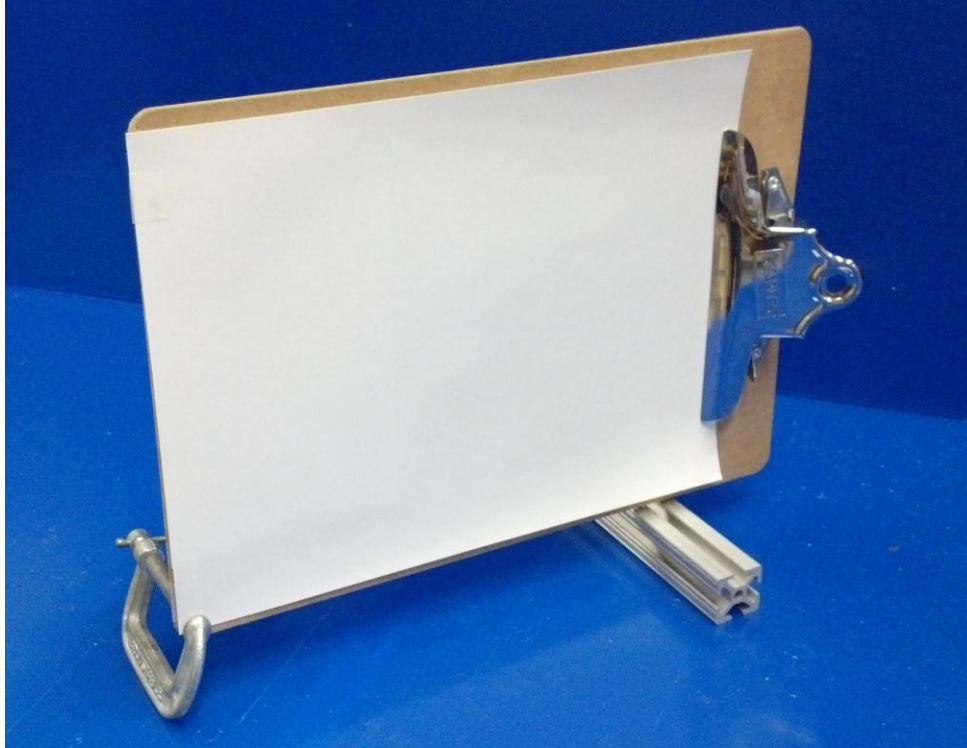
Figure 45: Screen used in z-type schlieren system
