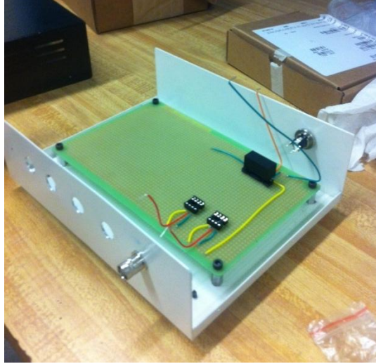
Figure 19: Project box holding transducer circuitry
