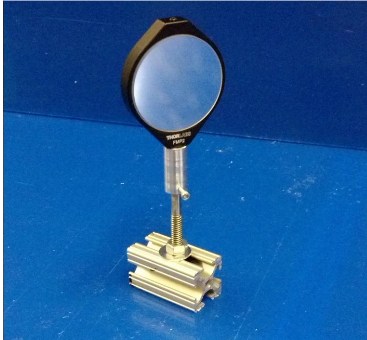
Figure 42: Concave mirror and mount used in z-type schlieren system
