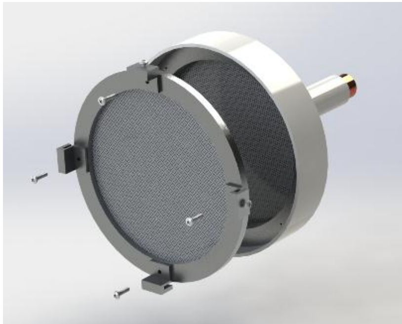
Figure 58: Initial design of air drier (outer diameter of funnel entrance (large end) is 13.13 inches for scale)
