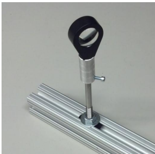
Figure 40: Condenser lens and mount used in z-type schlieren system
