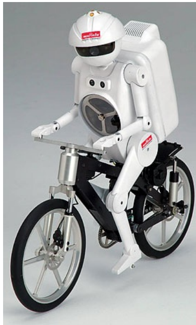
Figure 8: Murata Boy's flywheel embedded in its chest.
