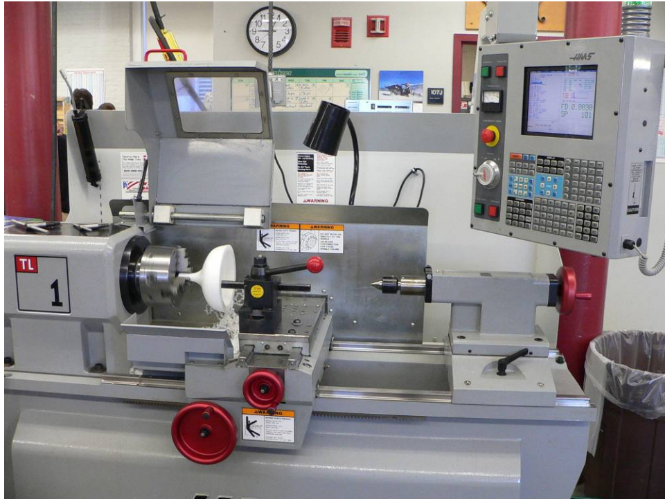
Figure 16 - Model 5 in TL-1 Interior Boring Operation
