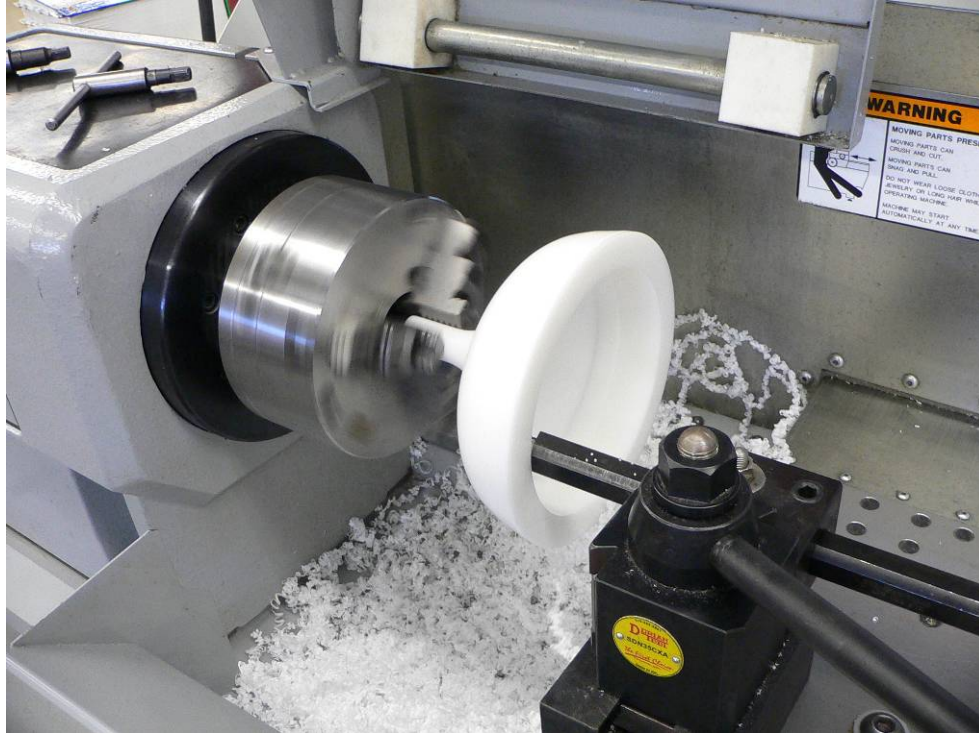
Figure 18 - Close-up of Interior Boring
