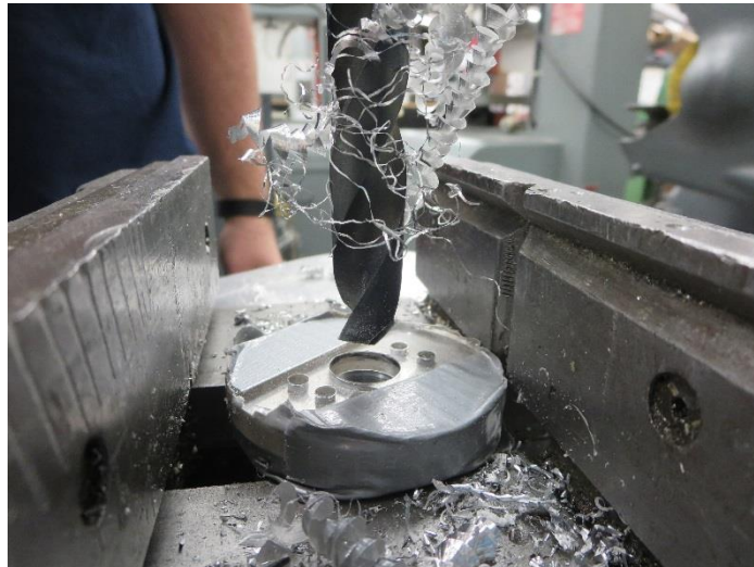
Figure 52 - Machining Motor Adapter Plate (Cheston)
