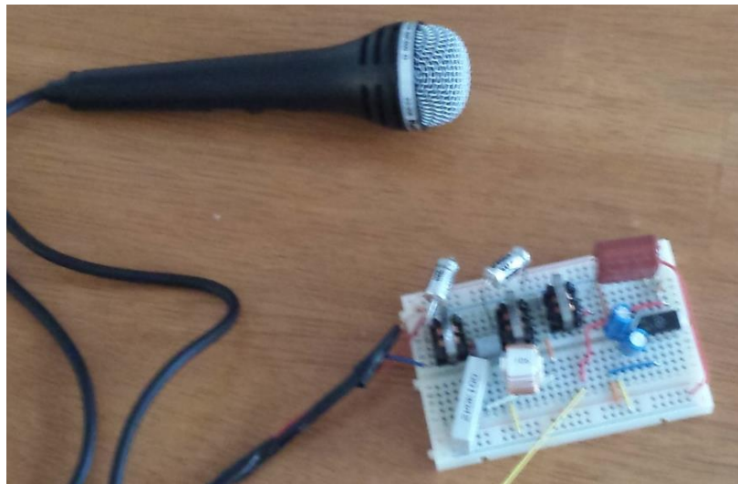
Figure 61: Buoy Relay Circuit Using a Breadboard
