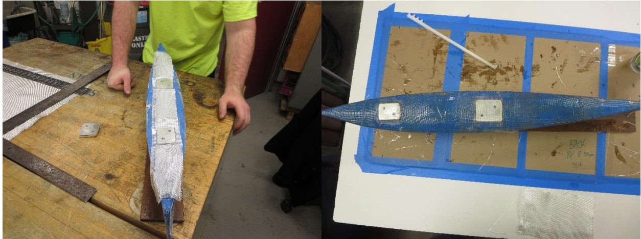
A. Fitting and planning fiberglass housing
