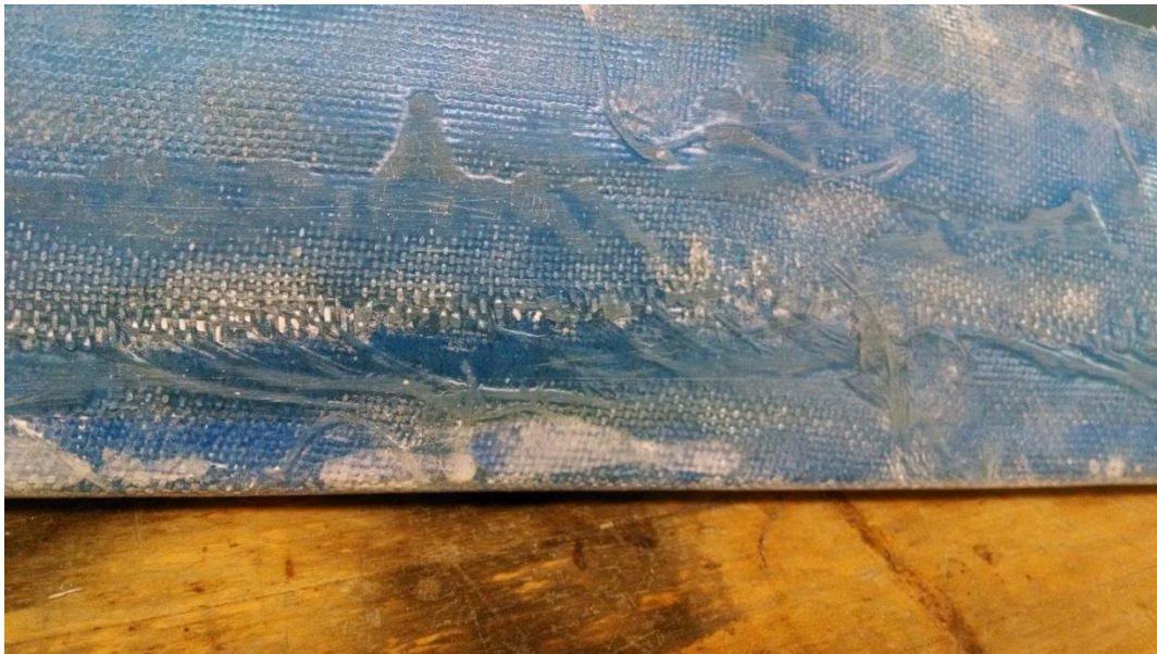
Figure 34 - Close up of sanded fiberglass threads.
