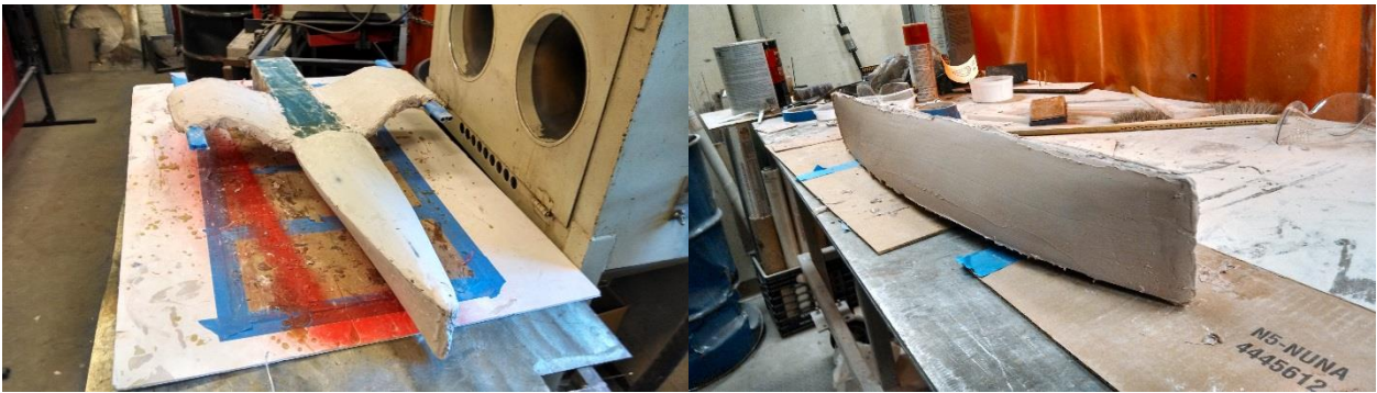
Figure 39 - Left: Center hull with Bondo caked on wings before sanding and sanded Bondo on bow. Right: Last layer of Bondo on one outrigger (no sanding).
