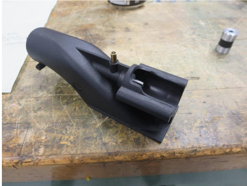
Figure 53 - Jet Drive Modified for Setscrew Access (Cheston)
