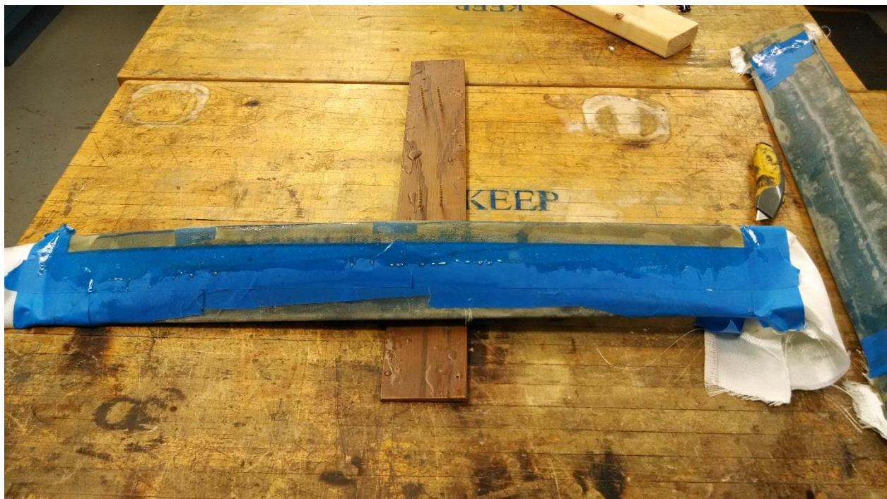
Figure 36 - Alternate pre-stretched fiberglass technique.
