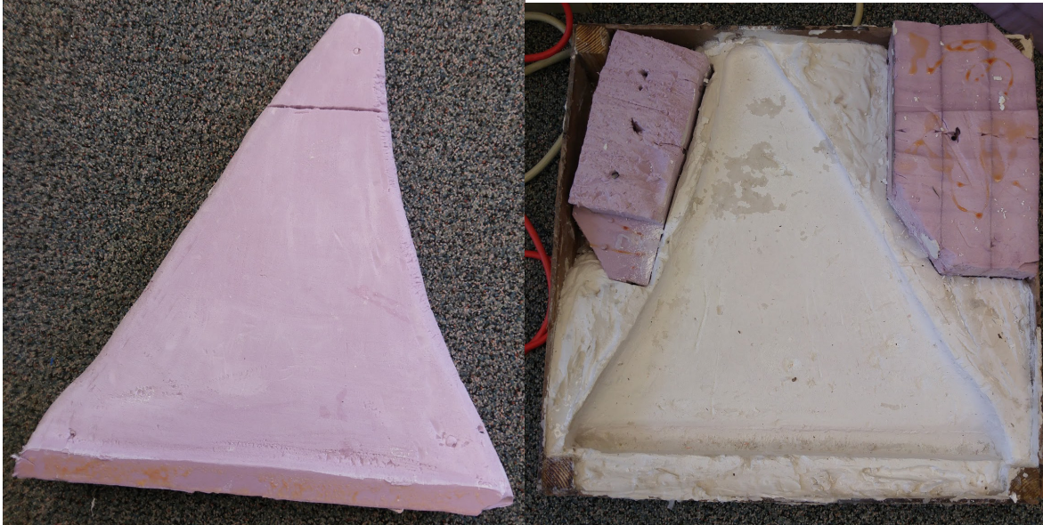
FIGURE 36: FOAM POSITIVE AND PLASTER NEGATIVE MOLD
