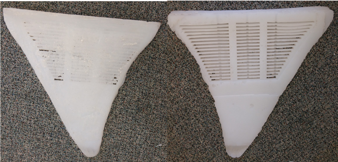
FIGURE 42: FAILED WING - SHALLOW CHANNELS
