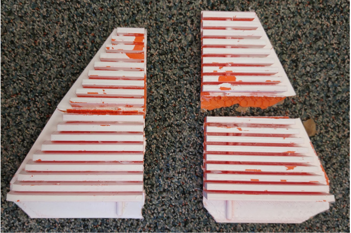
FIGURE 39: BROKEN CHANNEL INSERTS
