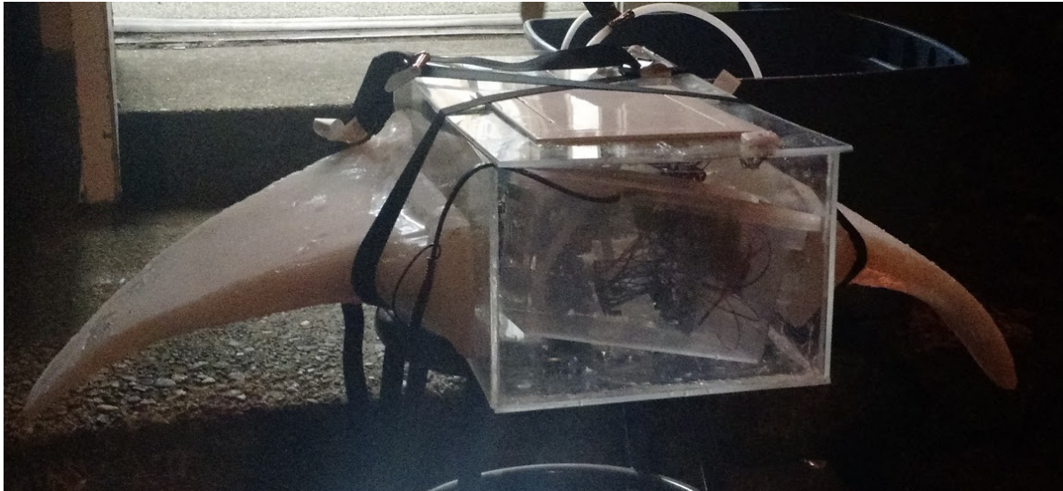
FIGURE 52: COMPLETED ROBOT WITH ACTUATED FINS
