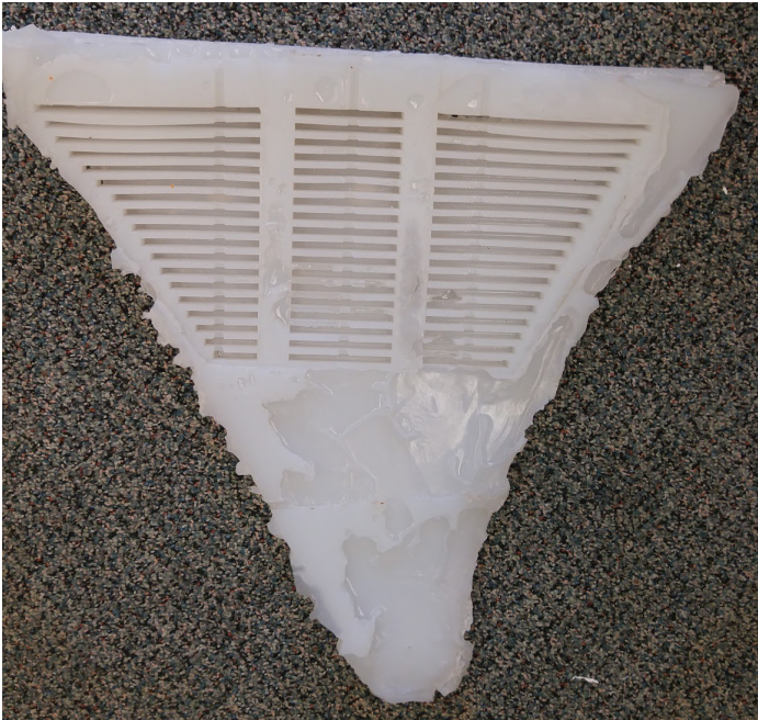
FIGURE 41: FAILED FIN - SILICONE BUBBLING
