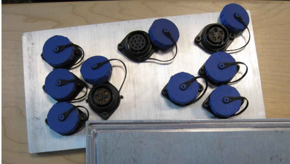
Figure 35: 5 and 12 Pin WEIPU Connectors.
