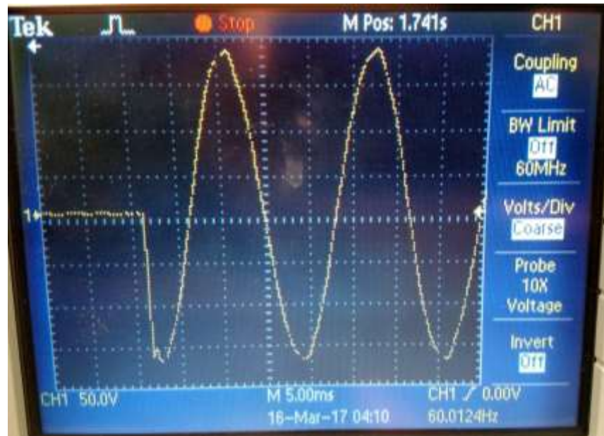
Figure 50. Electronic Breaker Transient Testing - Breaker Closing and Restoring Power
