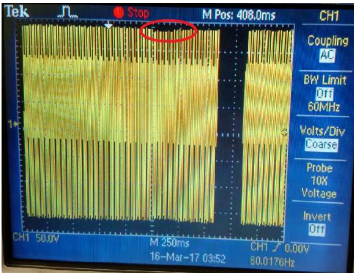
Figure 47. On-Grid Voltage Sag Caused by Motor Operation
