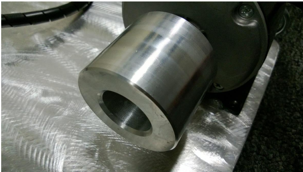
Figure 21 – Photograph of aluminum idler attached to DC motor
