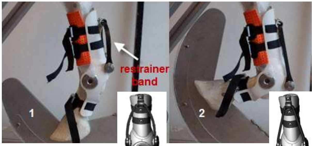
Figure 20 – Demonstration of the slack problem of restrainer band during flexion motion of horse forelimb.
