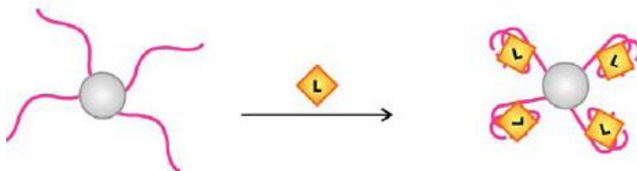
Figure 8. Schematic of Quantum Dot Sensor Utilizing Charge Transfer Quenching (Mok et al.)
