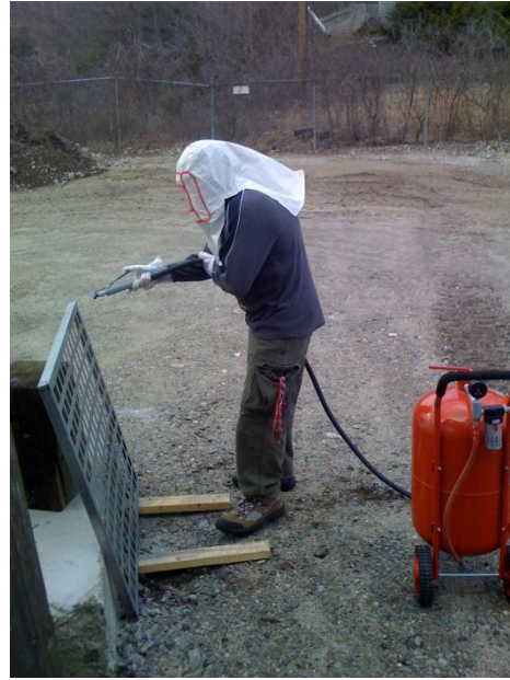
Figure 7- Glass beading a frame
