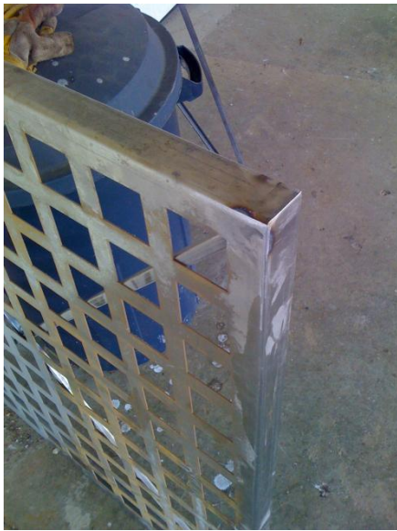
Figure 4- Welded corners ground smooth
