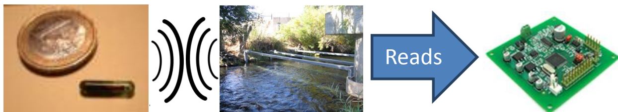
Figure 1.3-2 RFID concept diagram showing the tag, on the left, that would be inserted into the fish in order to communicate with the antenna array which is in the center and the reader, the photo on the right, receives the transmitted information. [13]
