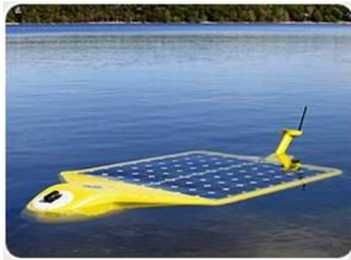
Figure 2.2-11 RPI underwater robot operated by solar panels on the surface of the water. The PVs are surrounded by the yellow framing of the robot.
