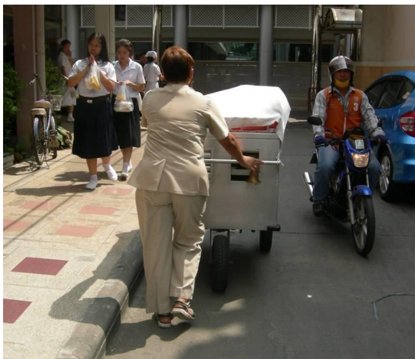
Figure 18: Trolley's Third Wheel that Inhibits the Operator's Ability to Push the Trolley
