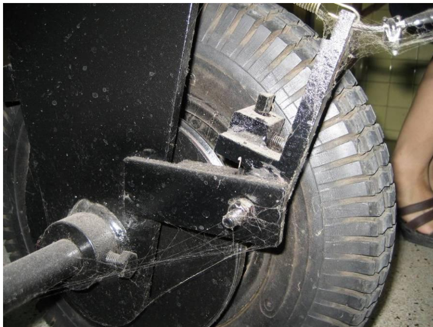
Figure 25: Brake on a Current Trolley
