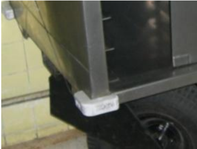
Figure 20: Bumpers on a Current Trolley
