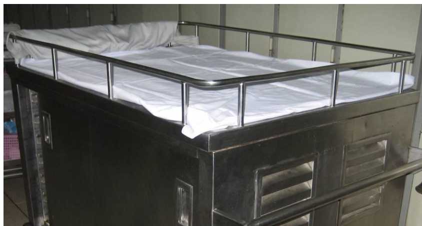
Figure 23: Containment Rack on a Current Trolley
