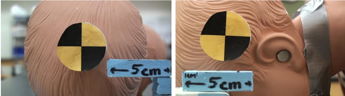
Figure 38. Displacement in the middle and side of the head determined from the fiducial markers' coordinates
