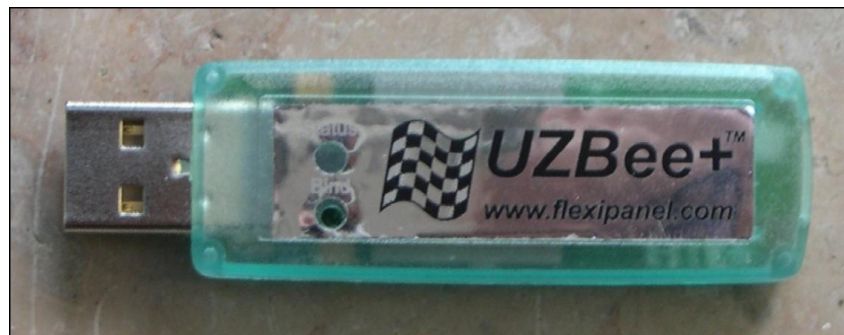
Figure 24: This is a 802.15.4 UZBee + dongle (from [16]).
