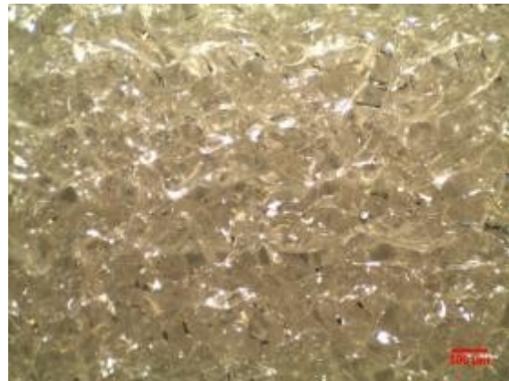
Figure 15 – Close up image of scaffold printed with 200µm nozzle with stretch
