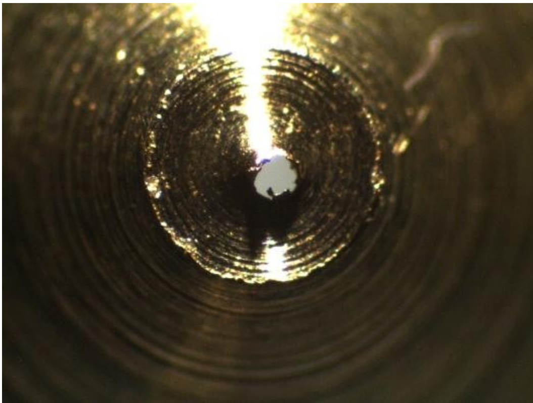
Custom 250 \mu m Nominal Bore Nozzle # 2 – Raw Image @ 35x – Bad Nozzle, Not Used
