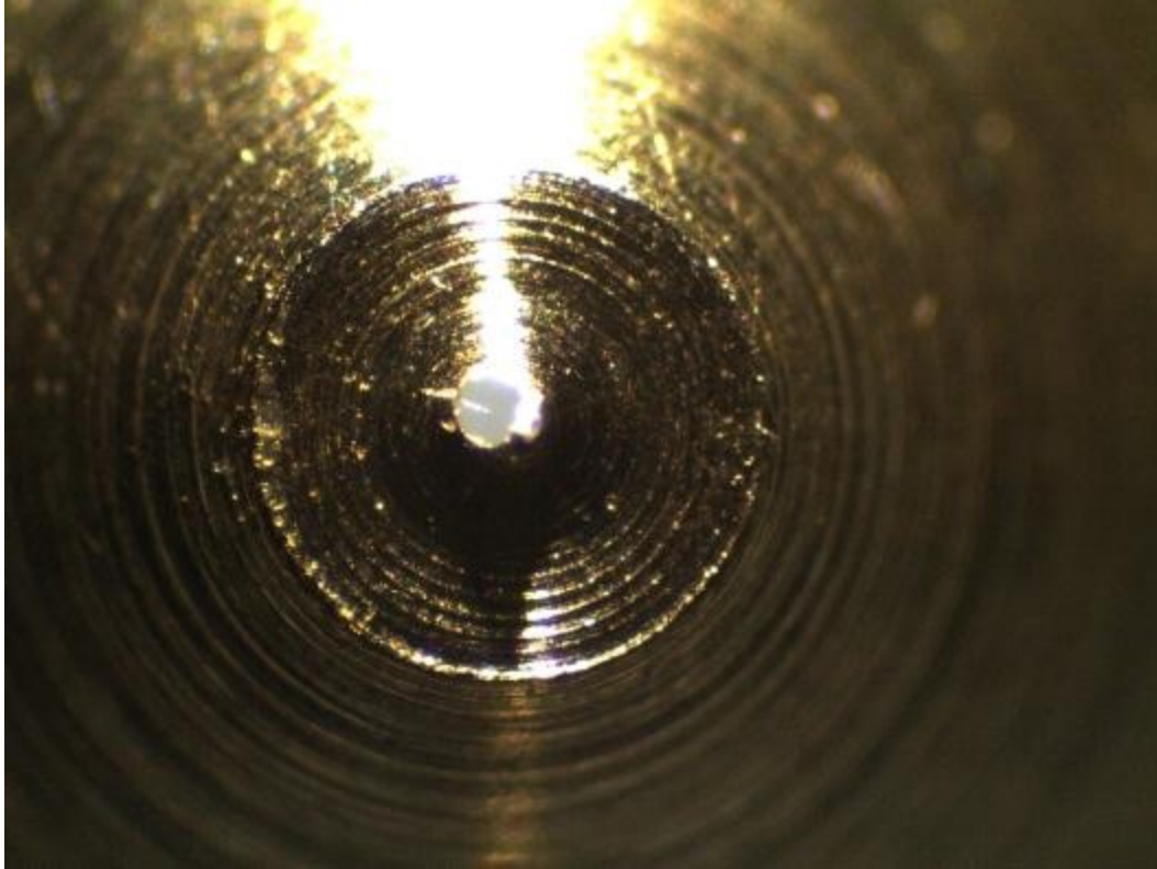
Custom 200 \mu m Nominal Bore Nozzle # 2 – Raw Image @ 35x – Bad Nozzle, Not Used
