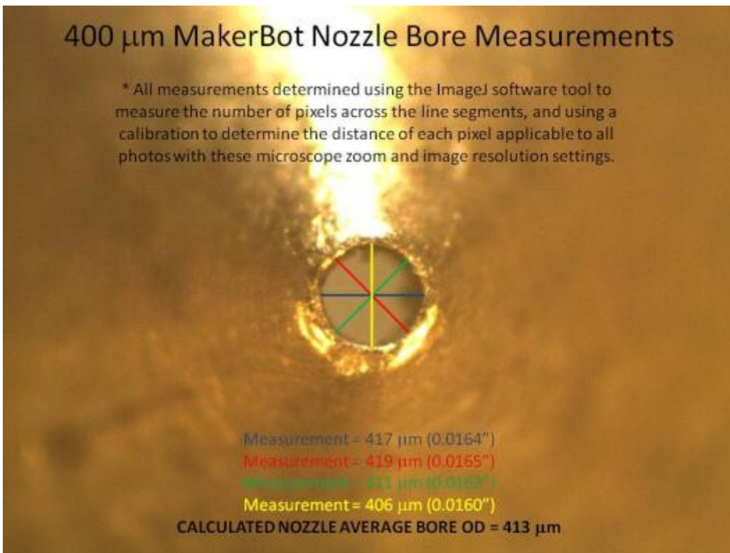
Measurements Using ImageJ Software – MakerBot Replicator Nozzle 1 – 400µm Nominal Bore
