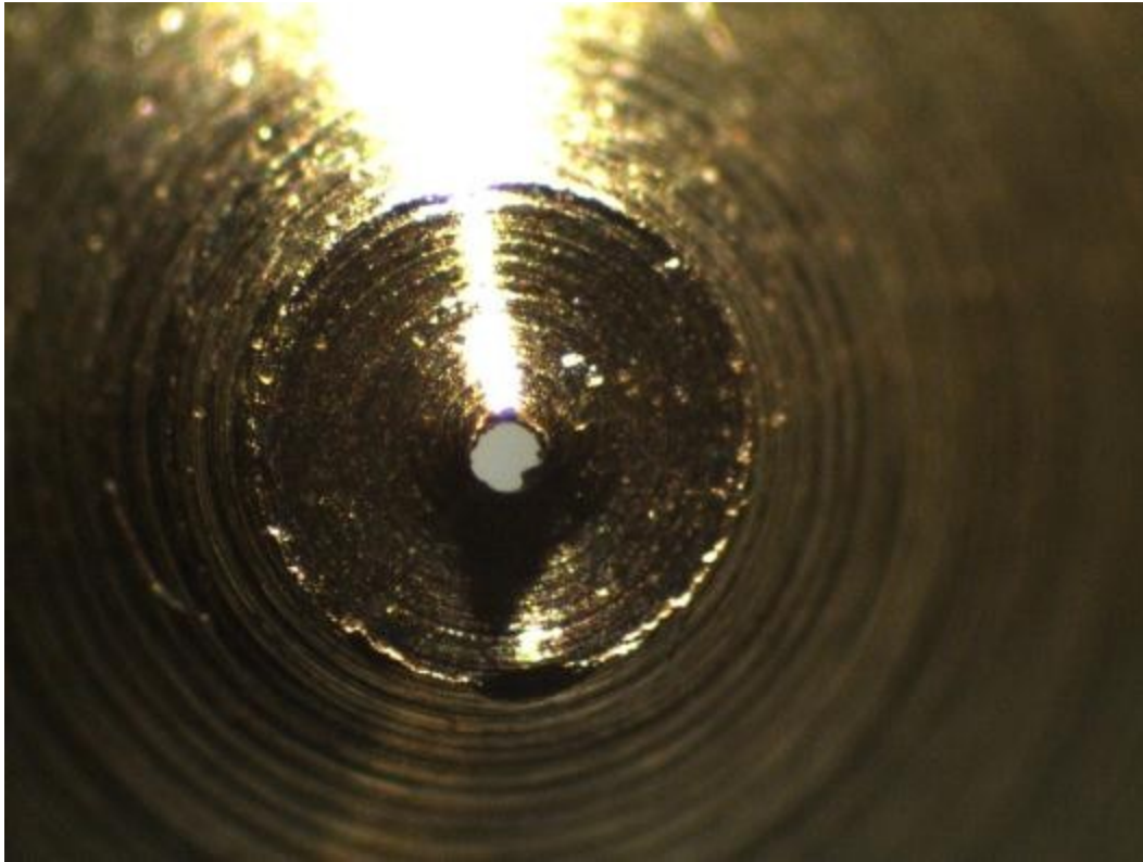
Custom 200µm Nominal Bore Nozzle # 1 – Raw Image @ 35x – Good Nozzle For Testing
