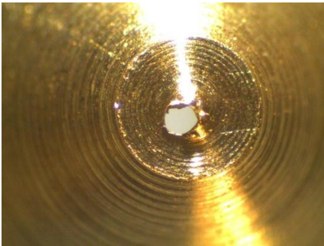
Custom 300 \mu\text{m} Nominal Bore Nozzle # 1 – Raw Image @ 35x – Bad Nozzle, Not Used
