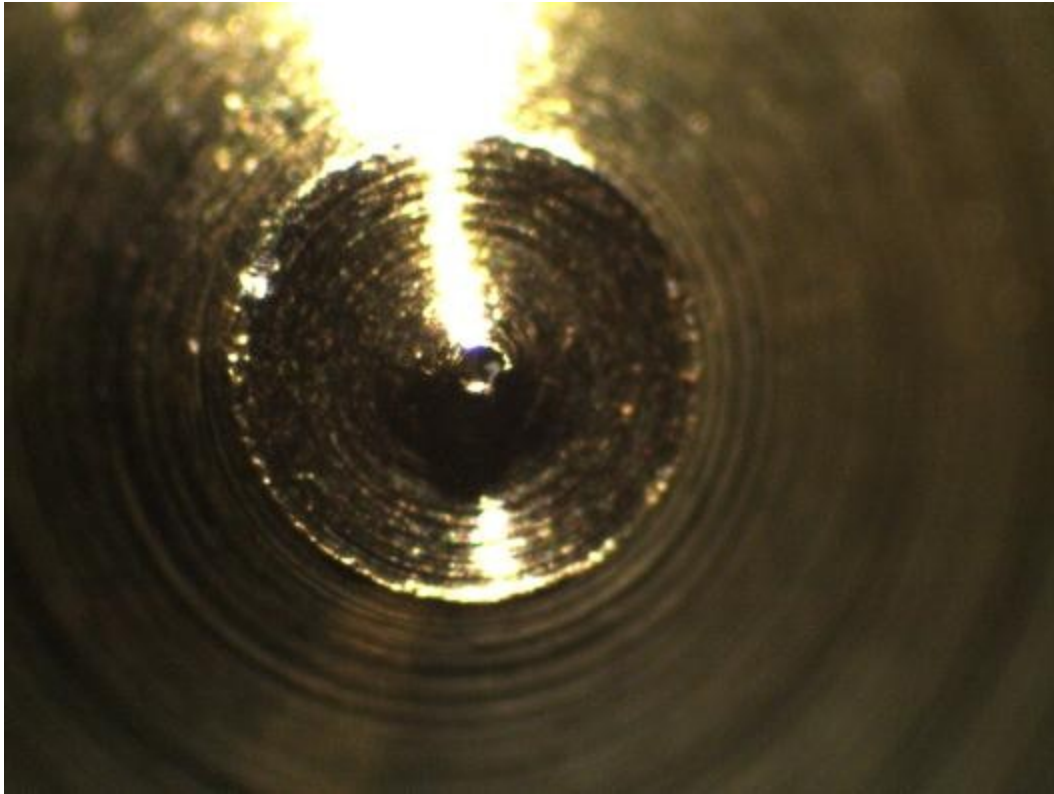
Custom 150µm Nominal Bore Nozzle # 1 – Raw Image @ 35x – Bad Nozzle, Not Used
