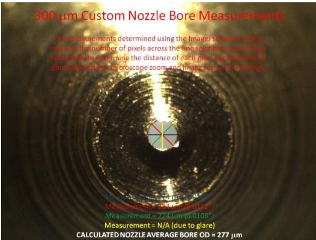
Measurements Using ImageJ Software – Custom 300µm Nominal Bore Nozzle # 2
