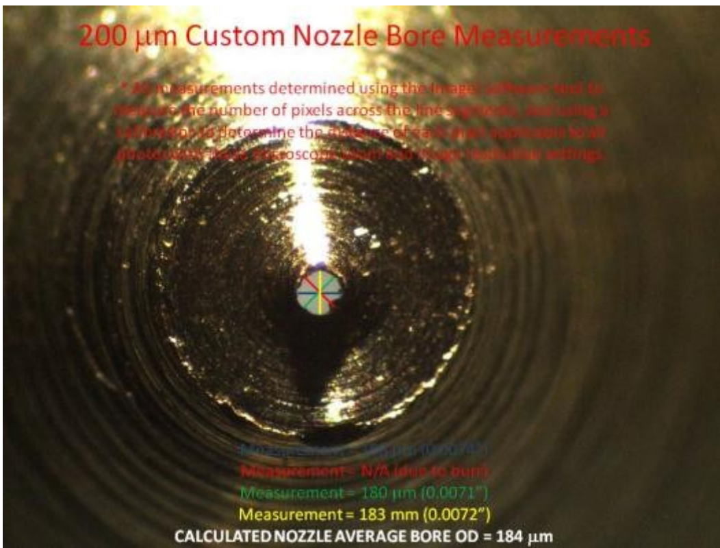
Measurements Using ImageJ Software – Custom 200µm Nominal Bore Nozzle # 1
