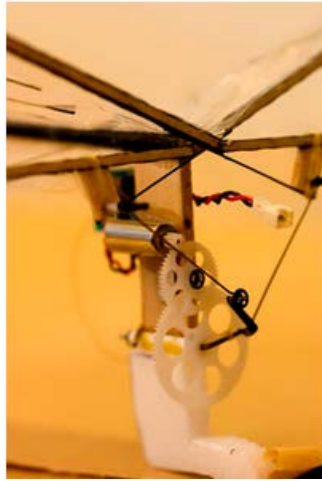
Figure 3: Delfly I Drivetrain ( Bruggeman, B. 2010 )
