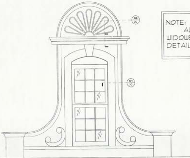
ELEVATION SCALE: 1" = 1'-0" WIDOW TYPE (W3) MOUL. REF.: 5/ALL4
