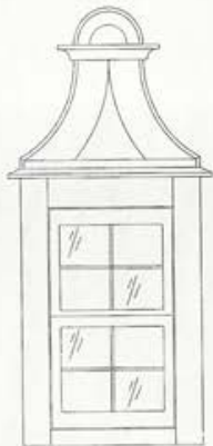
ELEVATION SCALE: 1" = 1'-0" WIDOW TYPE (W4) MOUL. REF.: 2/ALL1
