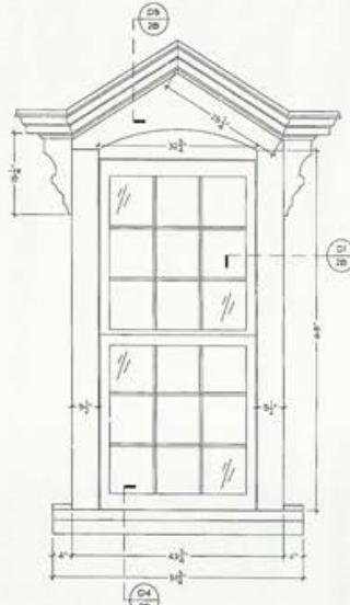
ELEVATION SCALE: 1" = 1'-0" MCK. REF.: 5/14.2 WINDOW TYPE (W2)
