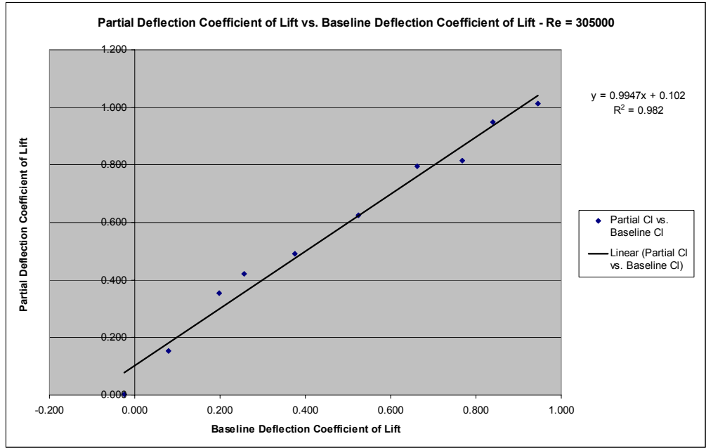
Figure 43: Partial Deflection Coefficient of Lift vs. Baseline Deflection Coefficient of Lift - Re = 305,000
