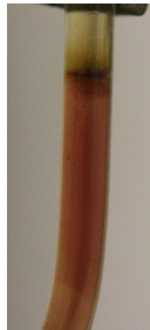
Figure 34 - Observation 3 Cathode Interphase: Continued diffusion of protein through interface
