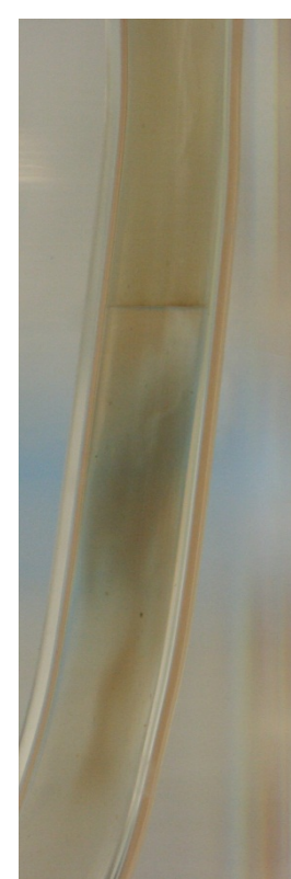
Figure 69 - Observation 2 Cathode Interphase: Protein continues to diffuse through interface boundary
