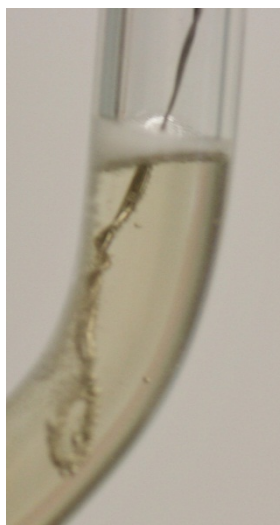
Figure 74 - Observation 1 Cathode: Fizzing on electrode
