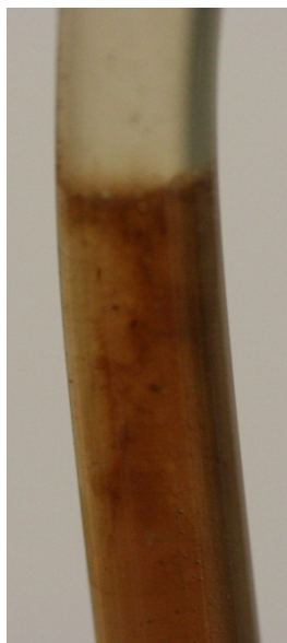
Figure 30 - Observation 5 Anode Interphase: Formation of dark cloud under the interface
