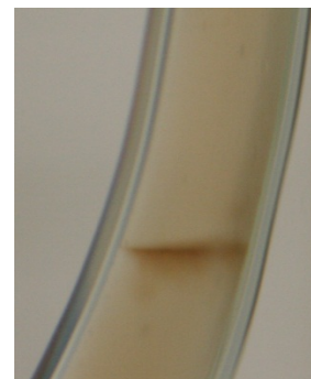
Figure 55 - Observation 1 Cathode Interface: Dark band formation due to inhibition of protein migration and establishment of new equilibrium
