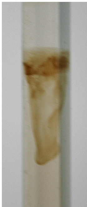
Figure 16 - Observation 4 Anode Interphase: Diffusion cloud has now moved under the interface
