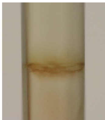
Figure 24 - Observation 4 Anode Interphase: Clearing out of protein at the interface, apparent disruption of the interface equilibrium
