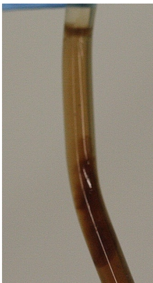
Figure 31 - Observation 1 Protein Accumulation: A dark region of protein formed quickly after the application of electrical current
