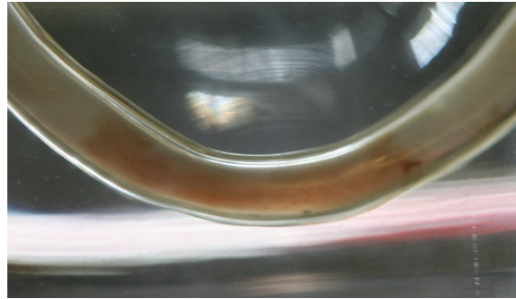
Figure 57 - Observation 3 Protein Accumulation: Protein cloud condensed and began to migrate towards the cathode
