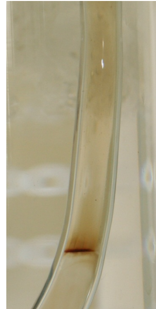
Figure 56 - Observation 3 Cathode Interface: Dark band at interface remains, heavy diffusion through interface into top phase
