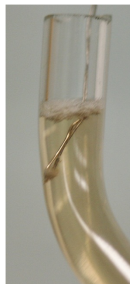
Figure 75 - Observation 1 Anode: Protein accumulation observed as small white solid on electrode
