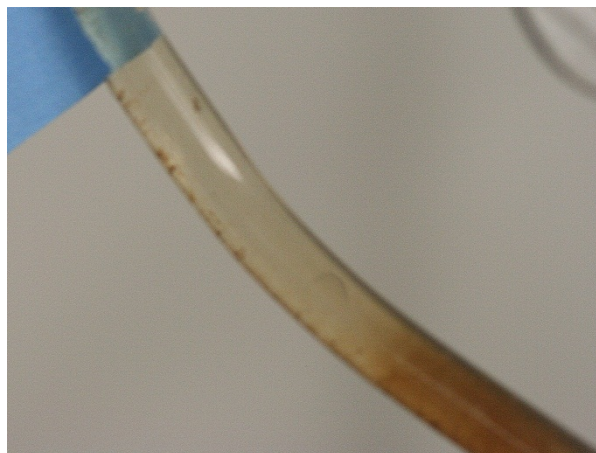
Figure 44 - Observation 2 Protein Cloud: Continued darkening of the protein cloud observed with rapid migration towards the cathode
