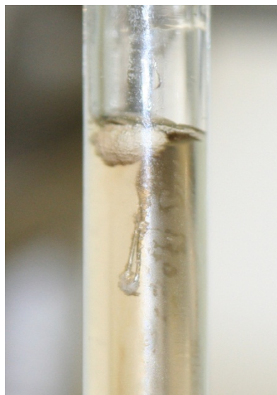
Figure 65 - Observation 1 Anode: Protein precipitation
