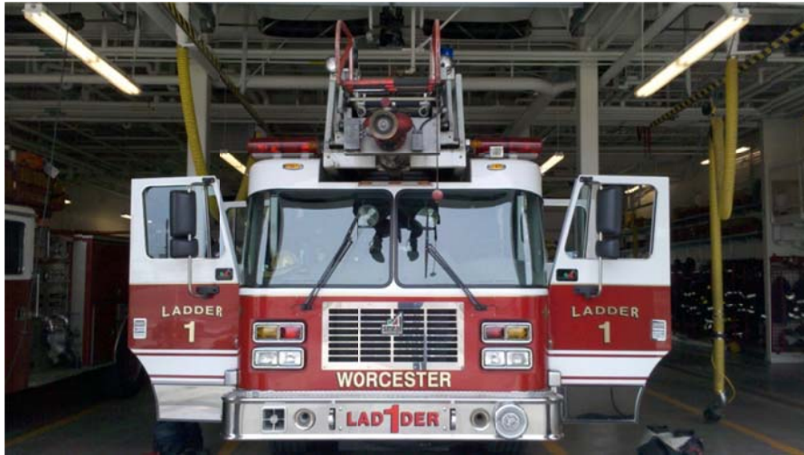
Figure 43: Worcester Ladder 1 with electronic siren, Horns, and mechanical Federal siren
