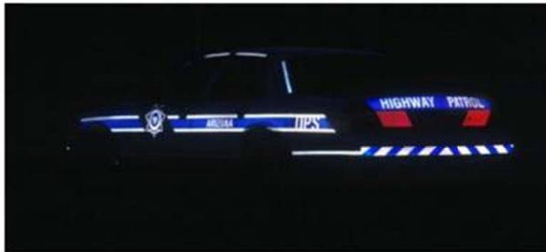
Figure 20: The effectiveness of retro-reflective tape. Note the use of text, symbols, colors, and patterns to clearly profile the car
