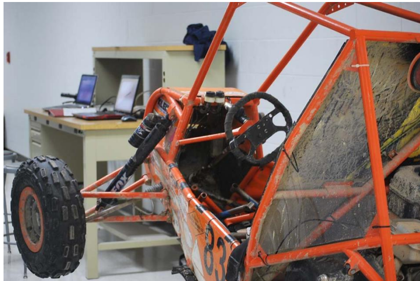
Figure 8 RIT's 2016 Vehicle Showing Double A-Arm in the Front Suspension
