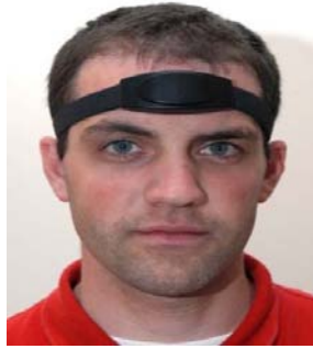
Sample of the ABS wireless physiological sensor.
