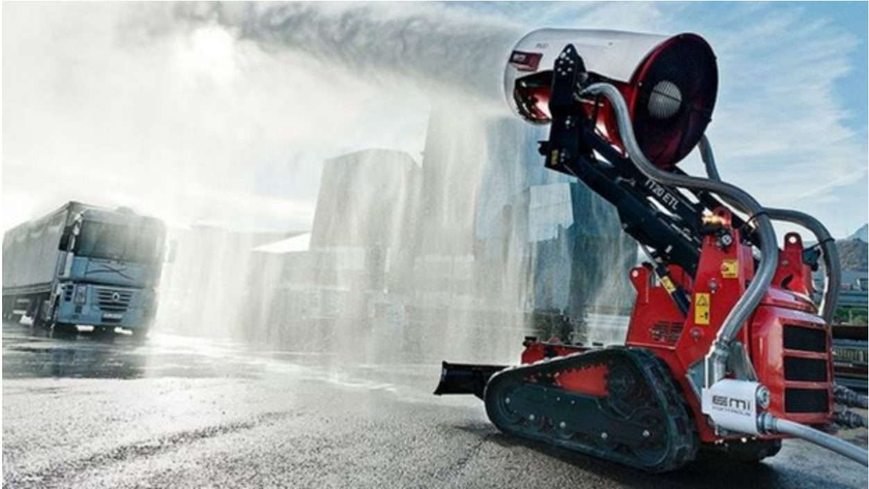
Figure 2. The water cannon is spraying mist instead of a focused stream (Bharat, 2015).
