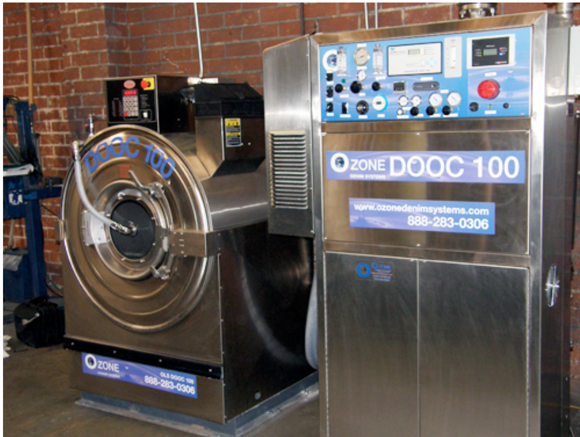
Figure 11- Ozone washing machines reduce moisture content in the linens, therefore the dry time is less than using a standard dryer.
