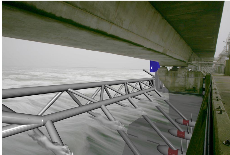
Figure 44: T200 Turbine in Oosterschelde, Netherlands
